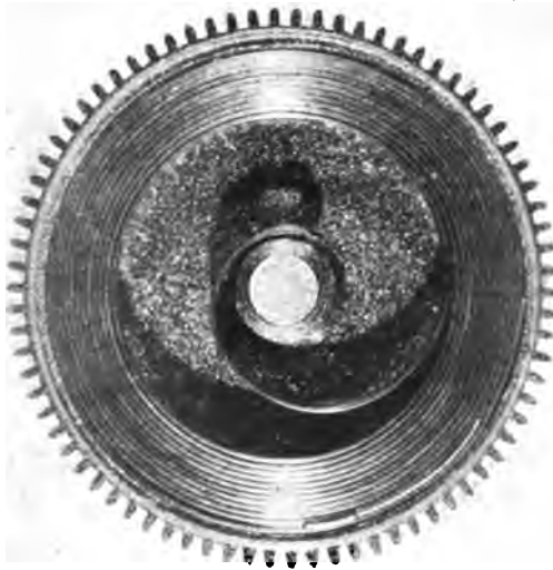
THE MAINSPRING, COILED IN THE "BARREL," IS THE POWER THAT DRIVES THE WATCH. (Magnified about five times.)
